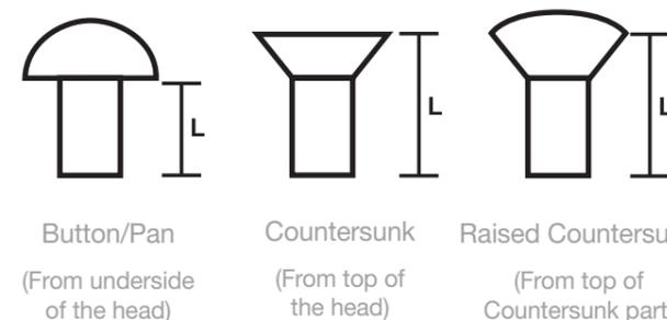
Button/Pan (From underside of the head)      Countersunk (From top of the head)      Raised Countersunk (From top of Countersunk part)
